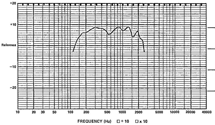
Figure 14. Frequency Response of Quad-Manifolded Mid-Bass Drivers (1 w @ 1 m; 100-dB Reference).
