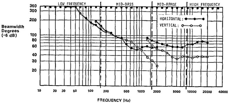
Figure 21. Beamwidth of MT-4 Loudspeaker System.
