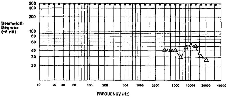
Figure 7. Beamwidth Plot of Typical 49mm Throat Feeding 40-degree Horn
