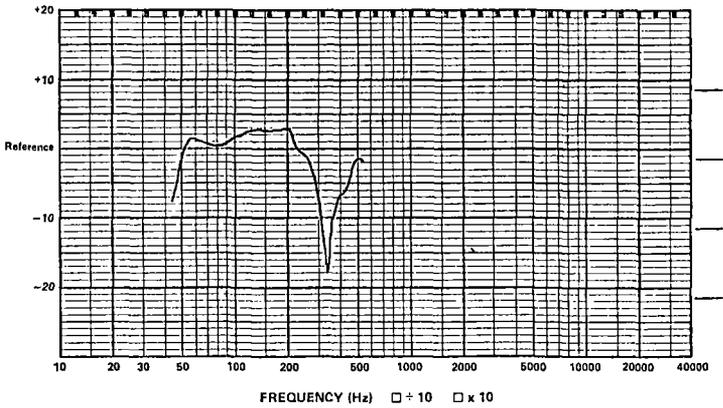
Figure 18. Frequency Response of Four Manifolded Woofers (1 w @ 1 m; 100-dB Reference).
