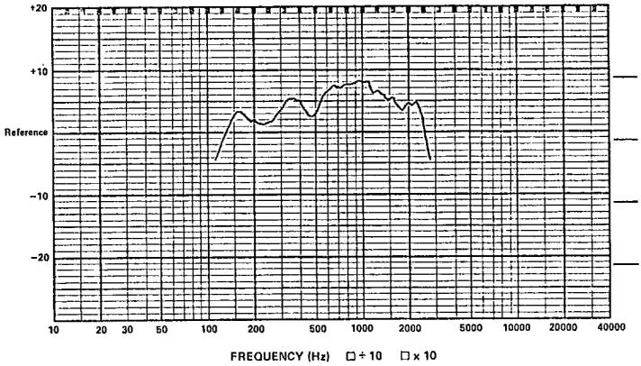
Figure 12. Frequency Response of Single Mid-Bass Driver (1 w @ 1 m; 100-dB Reference).
