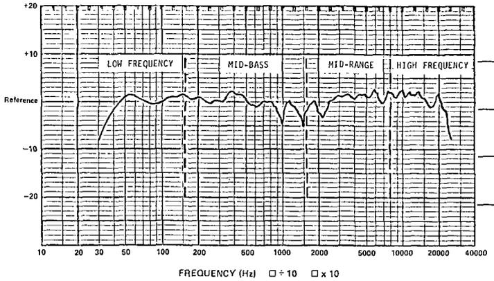
Figure 20. Frequency Response of MT-4 Loudspeaker System with Recommended Crossover, Equalization and Time Delay (10 w @ 3 m into Low-Frequency Section; 100-dB Reference).
