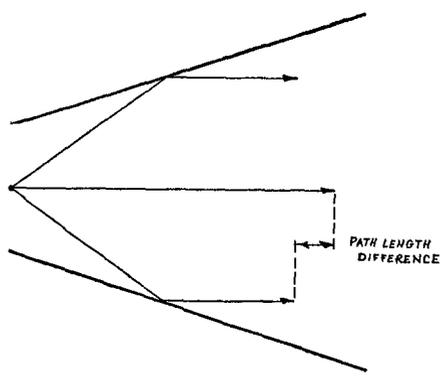
Figure 9. Path of rays in Horn Throat
