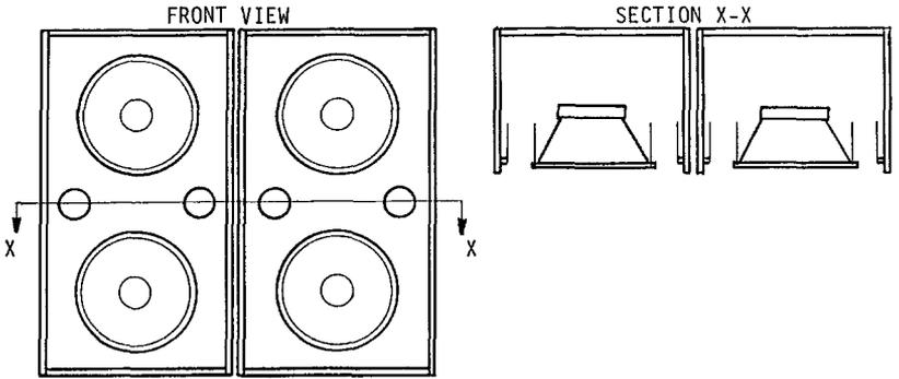
Figure 15. Four 46 cm Woofers Direct Radiating.
