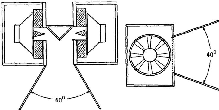
Figure 11. Two Mid-Bass Drivers Manifolded on a  $60^{\circ}$  X  $40^{\circ}$  Horn.
