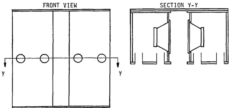
Figure 16. Four 46 cm Woofers Manifolded.
