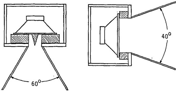
Figure 10. Single Mid-Bass Driver on a  $60^{\circ}$  X  $40^{\circ}$  Horn.
