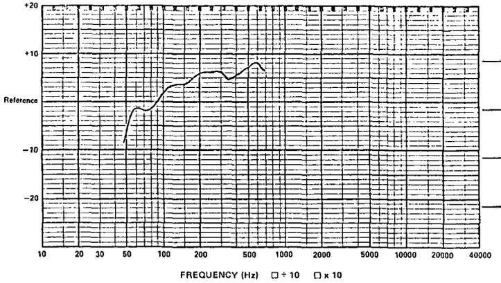
Figure 17. Frequency Response of Four Direct-Radiating Woofers. (1 w @ 1 m; 100-dB Reference).
