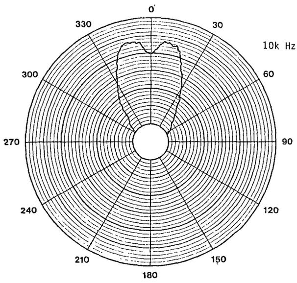
Figure 8. Polar Response, Typical 49mm Throat Feeding 40-degree Horn
