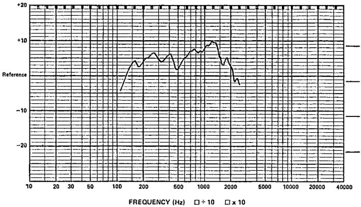
Figure 13. Frequency Response of Double-Manifolded Mid-Bass Drivers (1 w @ 1 m; 100-dB Reference).
