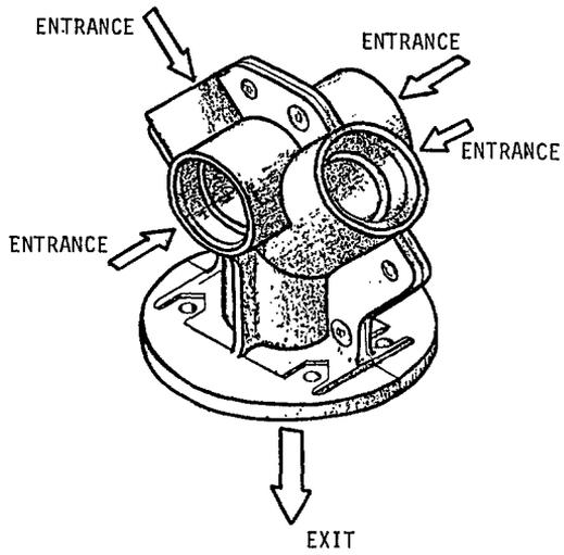
Figure 3. Manifold for Four Compression Drivers.
